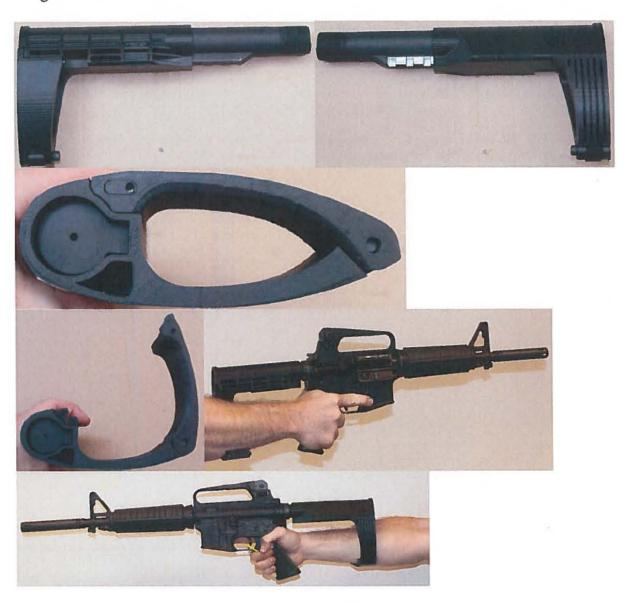
The FTISB examination found that when the sample is assembled as submitted; to an AR type pistol, a shooter would open the clamping feature of the sample, and place the resulting surface under his or her forearm while gripping the pistol's handgrip which offers the additional support. In this configuration, the device provides the shooter with additional support of the firearm while
