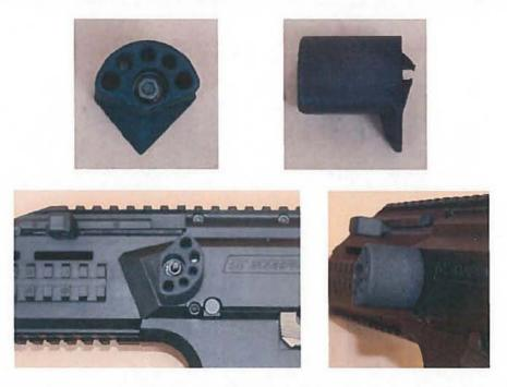
Sample 1 is an attachment to facilitate easier charging of the pistol along with acting as a thumb rest for the pistol. Sample 1 attaches directly to pistol's front sling swivel.
