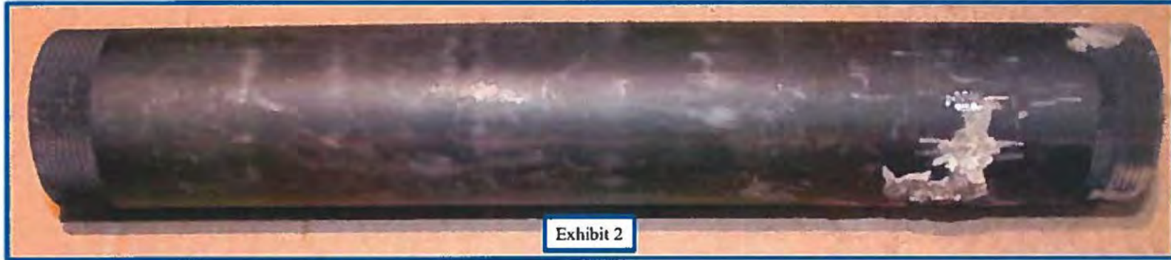
Exhibit 2 front view, note hole through central axis of device.
