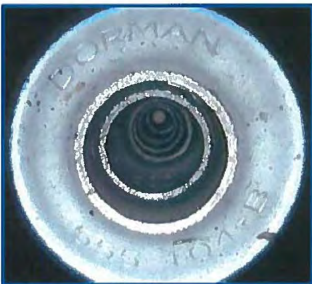
Exhibit 2 interior view showing improvised baffles constructed from freeze plugs.
